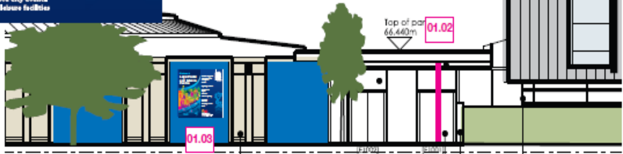
01.03 Listing wall sign Panel 1800mm square 30mm returns powder coated RAL5011 1mm stainless steel constructed box tray sign, printed graphics. Fixed to wall all fixings invisible.
